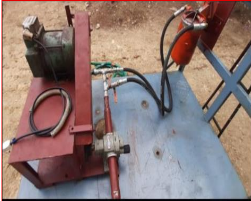
Bio-diesel Filtration unit with Single filter
